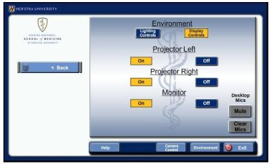
Select Display Controls to turn on or off projectors on confidence monitor. Here you can also choose to mute the goose neck microphones or clear them if multiple mics are on.
