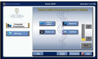
Once the system is ready, select Computer Presentation to use podium laptop or room computer. If using podium laptop, HDMI and VGA ports are located on podium, as shown in picture to the right. Select Sharelink as an option for wireless desktop sharing.
