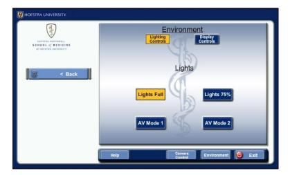
Press Environment button on bottom of screen to change lighting and display controls. Choose the lighting control that works best with your presentation.
