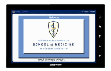
To get started press the tap panel. You can then choose any of the available sources by selecting the associated labels (VCR, DVD, PC'S, etc.). Select the source and a new touch panel page appears with additional source options. NOTE: the source volume is controlled by the buttons on the bezel, and environment screen.
