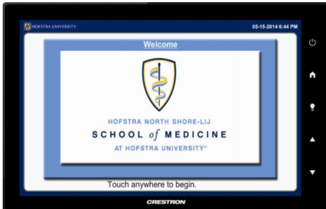
**To get started** press the touch panel. You can then choose any of the available sources by selecting the associated labels (VCR, DVD, PC'S, etc.). Select the source and a new touch panel page appears with additional source options. NOTE: the source volume is controlled by the buttons on the bezel, and environment screen.
