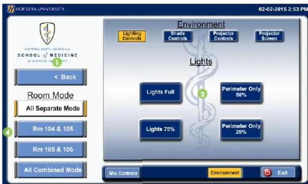
Press **Environment** to access **lighting controls, shade controls, projector controls, and the projector screen.**
