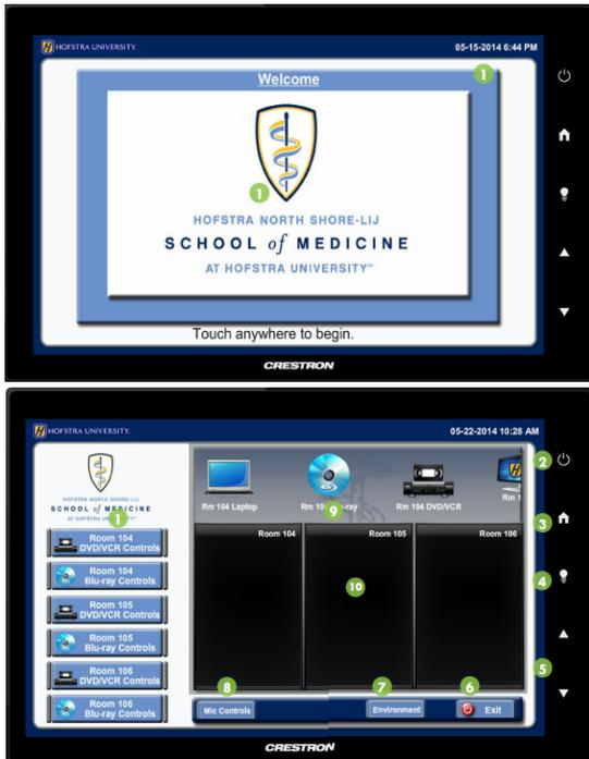
**To get started** press the touch panel. You can then choose any of the available sources (Laptop, Computer, DVD/VCR, etc.) displayed on the source selection bar by swiping left and right and then dragging it into the black space below the options. **NOTE:** The touch panel is programmed to control rooms based on the placement of the room dividers between rooms 104, 105, and 106.
